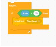
*Broadcast* is a very important piece of Scratch command code as it sends a message to some other part of the programme instructing it to implement a change. But for it to work, it has to have a corresponding *I receive* command that in this case will be positioned in the **Backdrop** script.
